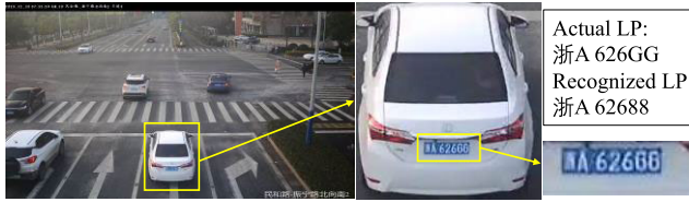
Fig. 6. Camera view of license plate recognition system and license plate recognition results. In this case, the letter ‘G’ is incorrectly recognized as the number ‘8’.
